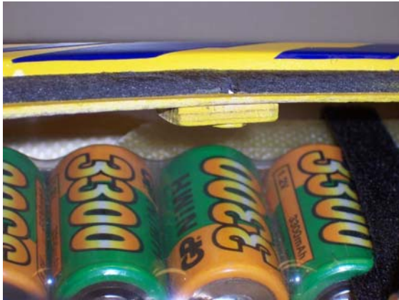
Photo 7: Small plywood supports and blindnuts glued to the underside of the deck ledge (Monohull)
