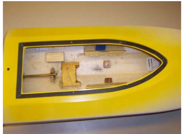
Photo 6: Foam placed around the deck, and corresponding hatch holes drilled through deck
