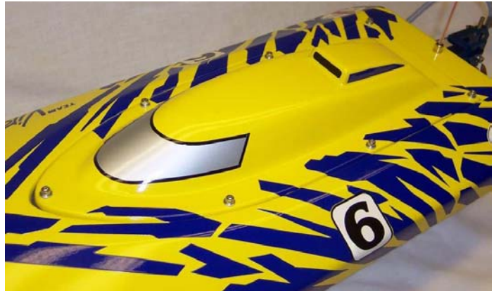
Photo 3: Monohull with screw-down hatch
