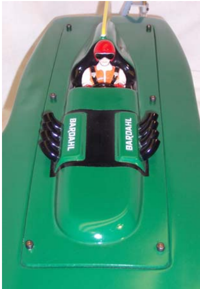
Photo 2: Hydroplane hull with screw-down hatch
