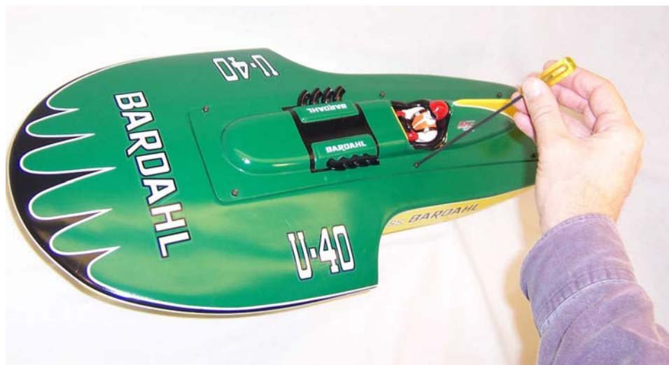
Photo 1: Screw-down hatches are easy, professional looking, and waterproof
