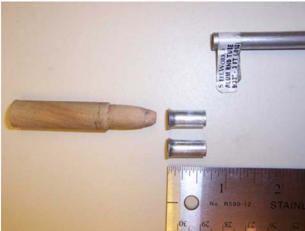
Photo 2: 9/32" aluminium tubing pieces and the dowel used to widen the ends
