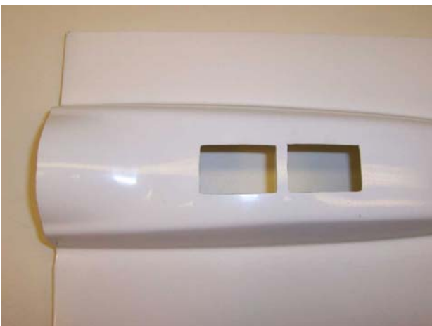
Photo 4: Hatch openings to accommodate "stacks"
