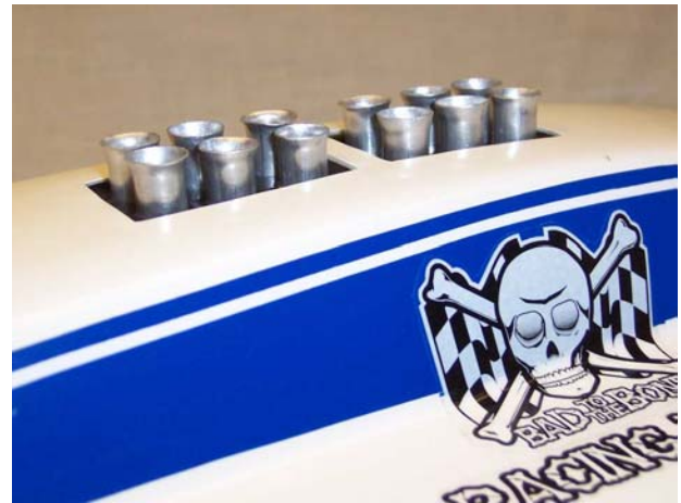
Photo 7: Stacks installed in hatch
